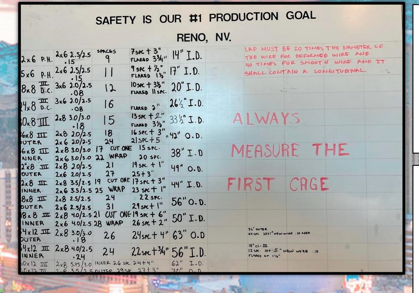
Posting Specifications for each size of pipe produced on the Cage Info Board has helped the Reno plant significantly reduce errors in production.
