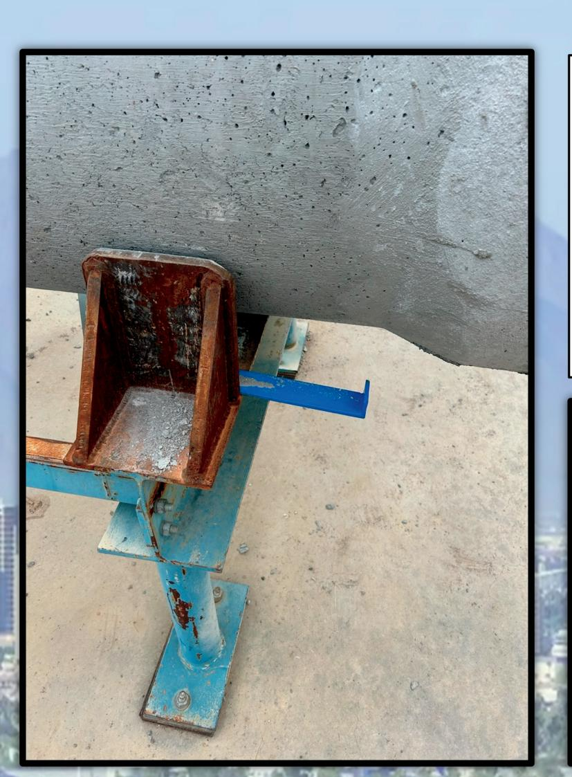
The D-Load Bar provides a simple but effective solution. Giving the loader a visual target for exact setting of the pipe, the first time.
