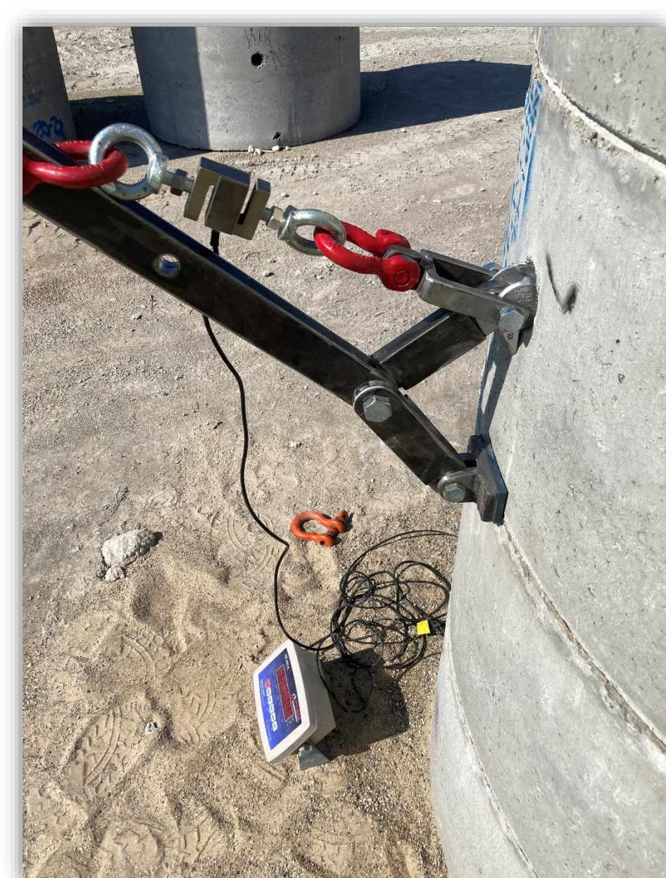
Works by leveraging off the product itself. Allows for testing in vertical or horizontal position and can be easily set to any angle that you'd like to test!
