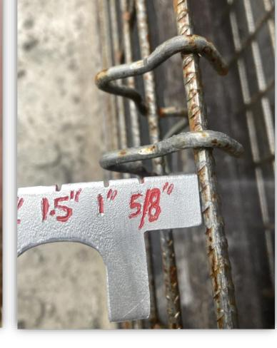
Production personnel can use this tool to make sure they have the correct rebar, anchors, stands, clips, and much more while preparing for production
