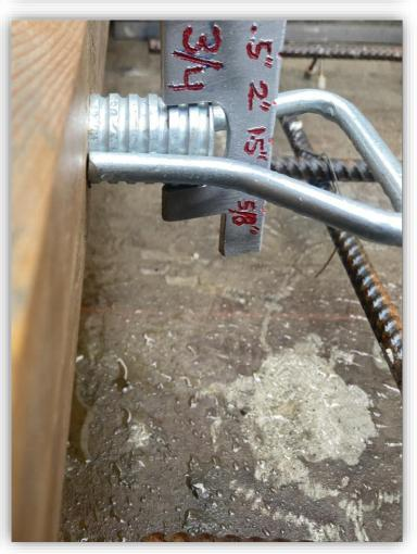
Then QC can use this tool to verify correct rebar sizes, wire spacing, concrete cover, anchor sizes, and lifting devices while preforming product pre-pour inspections
