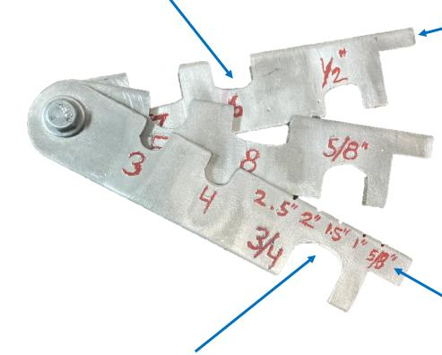
Cutouts sized to fit over common size threaded anchors to verify by external diameter when bolted to formwork (pre-production)
