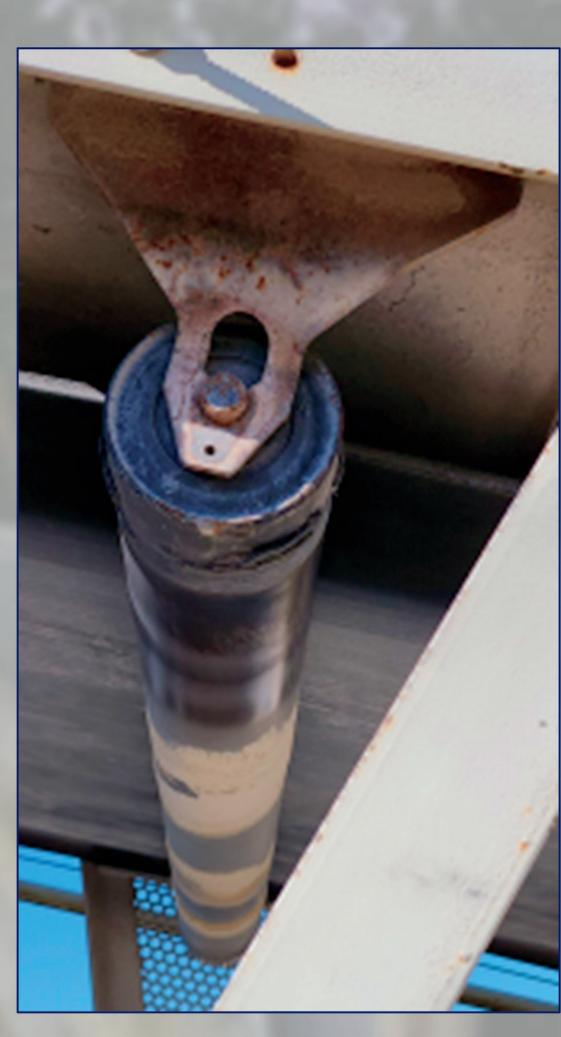
Every time we replace a return roller, the conveyor belt needs to be raised about one inch off the roller to have enough clearance. Since the belt is so long and heavy, we had to raise the belt with chain hoist to get that clearance. We fabricated a device with angle steel and all-threads to hold and raise the belt up enough to clear the roller off the bracket.
